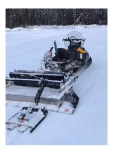
The **oil** should be checked periodically; the dipstick is the yellow cap under the cowling on the left side of the machine. Its tricky to lift off the plastic cowlings but don't force them they just lift up and out (yellow one first) and the black cowling has a single screw to release it.
