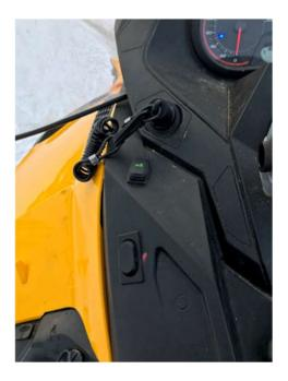
**Driving**: there are two forward and one reverse gears. When pulling a load always use first gear. The machine has three power modes; "eco", "standard" and "sport". The button on the left side of the panel that is labelled eco switches between modes. Eco saves gas but has limited power. Keep the machine in standard mode. Use "sport" mode if you are pulling through a lot of snow.
